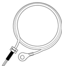
⑱ 72" Lower Cable
