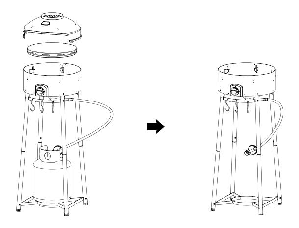
3. Unscrew the 2 hex screws that secure the legs to the body on the gas hose side of the oven. Then <u>CAREFULLY</u> flip your oven over.
