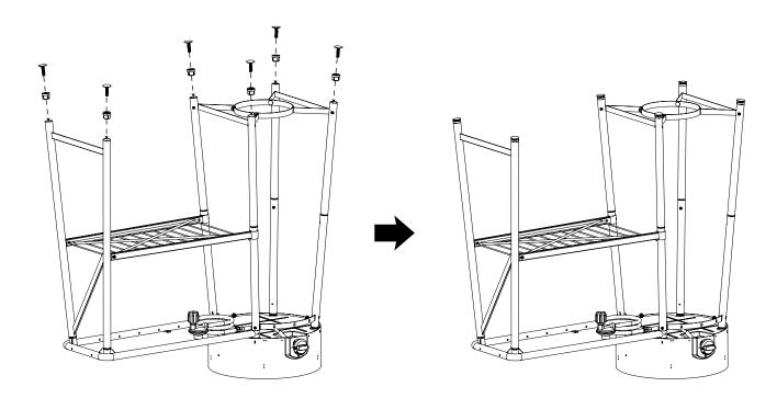
8. Attach interior and rear support bars. Align holes in tabs on wire shelf and U-channel with holes in interior support bar and use M6 carriage nuts and M6x12 carriage bolts to attach interior support bar. Then align holes in rear exterior leg and rear middle leg with rear support bar holes and secure with M5x15 screws.
