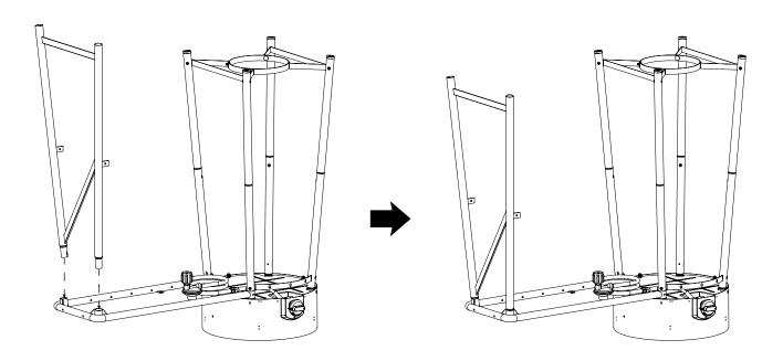
6. Detach the lower half of the legs on the side of the gas hose and slide the wire shelf end tubes over them, making sure the wire shelf is in the proper orientation. Replace the lower half of the leg kit legs and secure wire shelf to exterior leg tabs with M6x8 phillips head screws.
