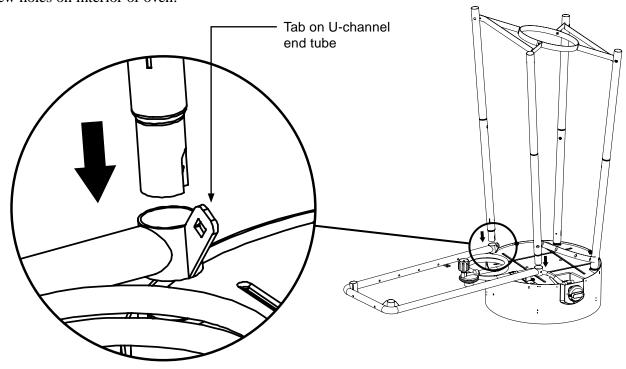
5. Insert exterior legs into the corresponding brackets just inside the U-channel, making sure the brackets extend away from the oven body and the tabs on the legs are facing inward toward the oven. Align the screw holes where the legs and brackets overlap and secure with M6x12 hex screws.
