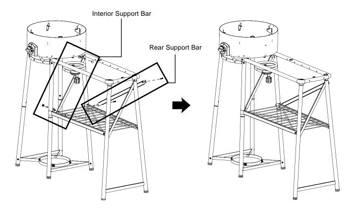
9. Insert M6x8 phillips head screws to lock U-channel and wire shelf into place. Make sure your U-channel and wire shelf are level, then insert M6x8 screws into the M6 nuts welded to the end tubes of the U-channel and wire shelf that capture the middle legs from the leg kit. Secure tightly to prevent
