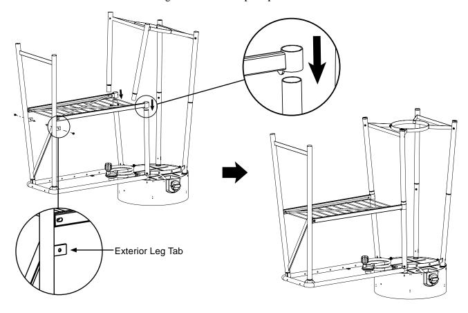
7. Using pliers, remove the plastic feet at the base of the leg kit legs. Replace feet with new plastic feet that came with your workstation. You should have 6 total: 4 for the existing leg kit legs and 2 for the exterior legs that came with your workstation. Now screw an elevator bolt into each foot and carefully flip the entire unit back over (You're almost done!)
