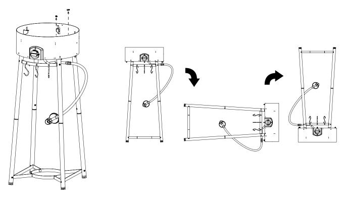
4. Remove the legs from the oven body on the gas hose side. Then align the U-channel end tubes with the legs on the side of the gas hose, making sure the tab on the U-channel end tube is facing away from the oven body, as shown below. Slide legs through U-channel end tubes and re-attach legs to oven body and secure with existing hex screws (you will need to turn oven onto its side to access body screw holes on interior of oven.
