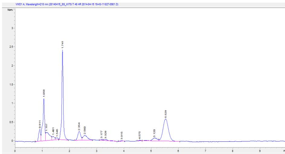
Figure 5: Sample chromatogram for Pill Terminator destruction kit containing morphine (retention time 4.6 min) at T=48h.
