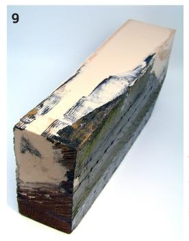
Same repair state as Photo 8. Note the line of holes that have been drilled along the crack. These were sized such that the mixer tip of a cartridge of SilverTip GelMagic adhesive could be seated in the hole allowing GelMagic to be injected into the crack. This both sealed the crack and bonded the two sides together. At this point all the strength has been returned to the beam.
