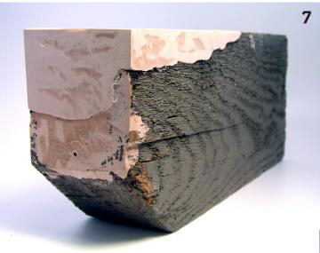
The plywood mold boards have now been removed and the SculpWood sanded to "clean it up" The edges on the sides and end of the beam exist because the beam was slightly concave. These will be "faired" in later using SculpWood Paste. Note the split in the forward part of the beam. This is the extension on the crack mentioned in Photo 1.
