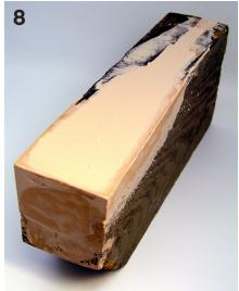
The slight recess in the top has been filled with SculpWood Paste using the newly formed edges as a guide. The side edges have been faired in.
