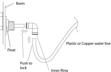
To release water line, push inner ring towards elbow and pull
