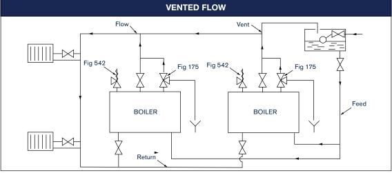
In both types of installation, there must be no isolating valve fitted between the Fig 175 and the boiler, vent pipe or drain.
