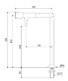
**Description**: Single Pillar tap with Twin outlets Removeable nozzles.
