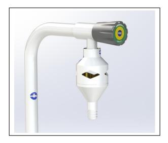
The product is designed specifically to protect the water supply against contamination from back siphonage within the laboratory environment. The nozzle must be permanently fitted to the outlet of the laboratory water tap with Loctite 648. The fitting of this nozzle will introduce the statutory air gap.
