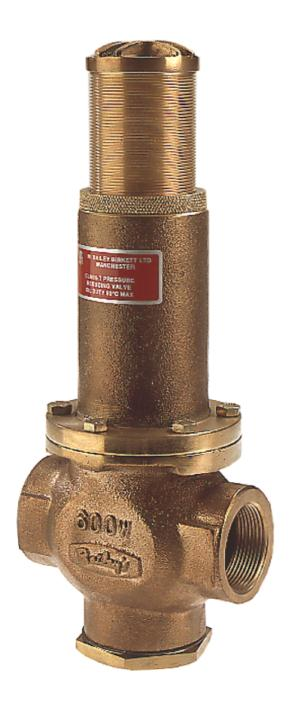
The Class T balanced direct acting pressure regulator is designed for use on installations that have varying inlet pressures and capacities, and require positive shut-off under "no flow" conditions. The standard valve is suitable for controlling air, gas and water. Alternative seals and diaphragms need to be fitted for oil duty.
