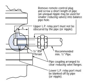
'A' dimension must be  $15/16" \pm 1/16"$  on all stainless steel valves or CS Fig 2046. All other valves with bronze pilot tops, the pipe should penetrate 1" minimum.
