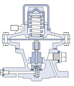
The standard 'G4' pilot top can reduce pressures down to 0.35 Barg (5 Psig). For pressures below this, a bronze low pressure pilot top can be fitted in place of the standard top. It is suitable for outlet pressures from 0.07 to 0.35 Barg (1 to 5 Psig) using the yellow spring. The low pressure top is available for fitting on to valve sizes 15 to 100mm ( $\frac{1}{2}$  to 4 inch), and a balance line should always be fitted to a low pressure top, on steam duty and never on gas duty.
