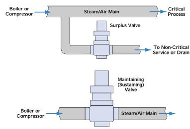
The 'G4 Maintaining' valve is designed to be installed in the main pipeline from the boiler or an air compressor (see figure 2), to maintain the pressure in the boiler or accumulator, thus preventing the boiler or accumulator from becoming exhausted.
