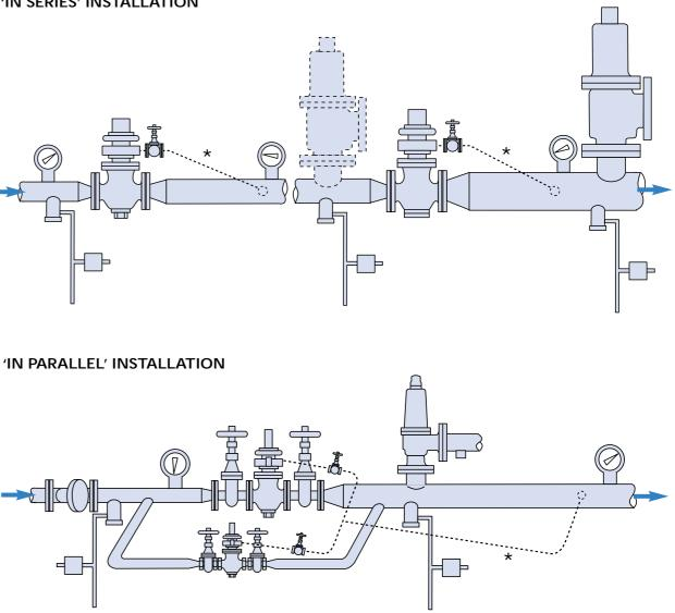
\*Balance lines are only required on some steam applications, they are not required on air/gas applications.
