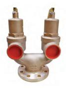
The NABIC 520 double spring safety valve. We keep the valve with the inlet flange un-drilled, this allows us to drill to client requirements. The 520 series has been designed primarily for use on unvented hot water heating systems, where a high capacity emergency steam relief capability is required.
