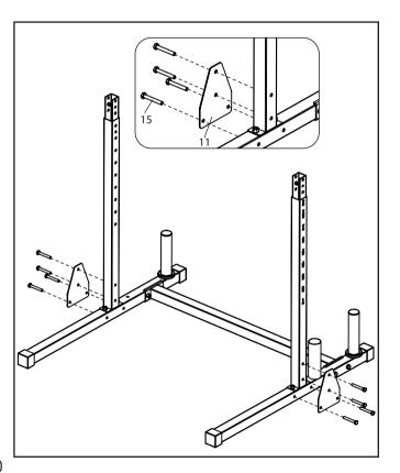
Slide Support Plate (11) onto M10X70mm Bolts (15), Secure with M10 Nuts (19).
