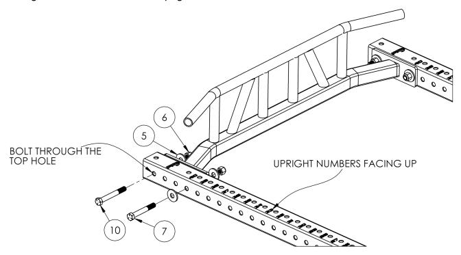
Figure 7: Attaching the Multi-Grip Bar to the Uprights
