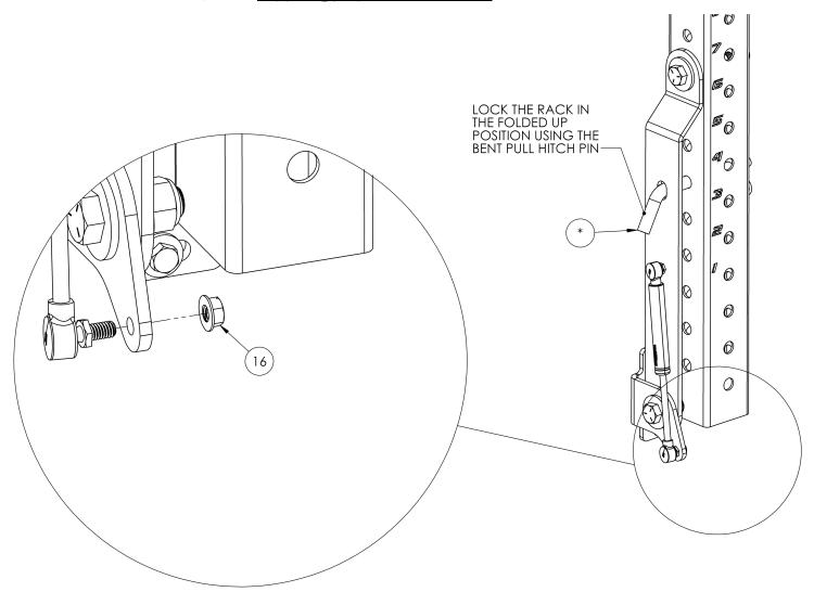
Figure 10: Attaching the Gas Shocks
