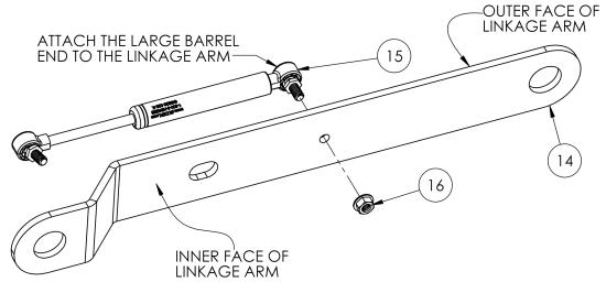
Figure 5: Attaching Gas Shocks to Linkage Arms
