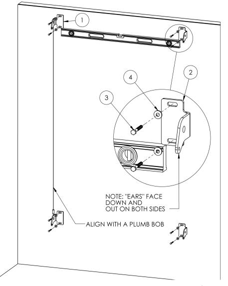
Figure 3: Installing the Wall Brackets with Lag Screws
