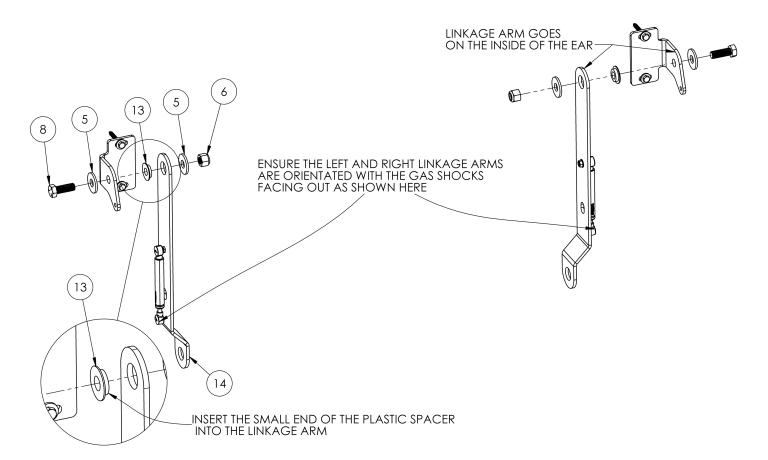
Figure 6: Bolting on the Linkage Arms
