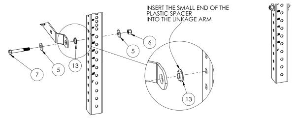
Figure 9: Bolting the Rack to the Lower Linkage Arms
