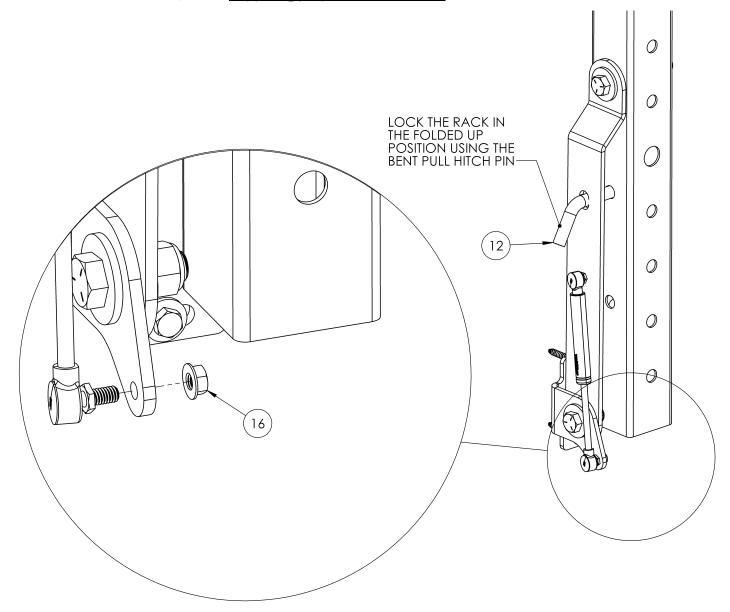
Figure 10: Attaching the Gas Shocks
