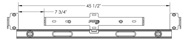
Figure 4: Stabilizer bracket vertical and horizontal alignment
