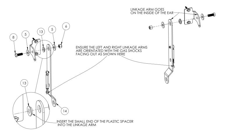
Figure 6: Bolting on the Linkage Arms
