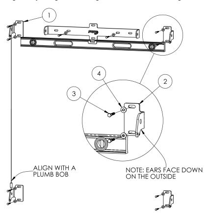
Figure 3: Installing the Wall Brackets with Lag Screws
