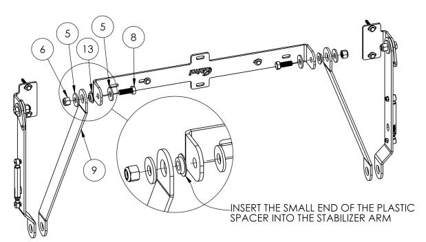
Figure 7: Attaching the Stabilizer Arms
