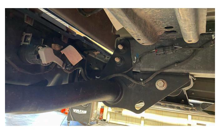
With the wiring separated the bumper assembly can now be removed. The receiver hitch and bumper are bolted into one assembly so only the frame bolt locations need to be loosened. If your truck is a Rubicon, the bed side rub rails and their frame support brackets will need to be removed prior to the other bumper mounting bolts. Fully separate and remove the Rubicon rub rails and brackets from the truck and detach from the main bumper corners.
