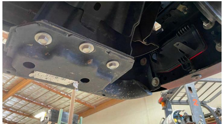
Unbolt and remove the original bumper from the truck via the 2 bolts under each frame rail and the 2 through. Leaving one through the frame on each side will support the bumper for final removal, we recommend 2 people to support and remove the bumper assembly.
