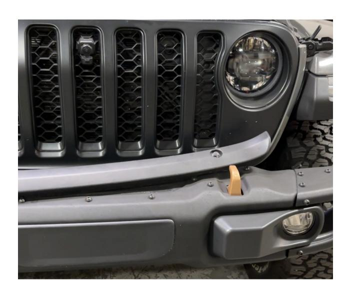
Disconnect the fog light wiring harness connector at the outer side of the passenger frame rail near the lower corner of the grille.
