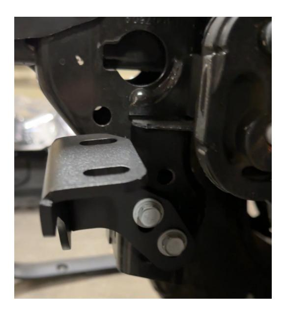
Next, mount the included winch plate support brackets to the bottom of the winch plate and down to the skid plate bolt locations on the lower frame 'tusks' from earlier. The included 3/8" hardware will secure the brackets to the bottom of the winch plate, the factory bolts will secure the brackets to the frame of the Jeep.
