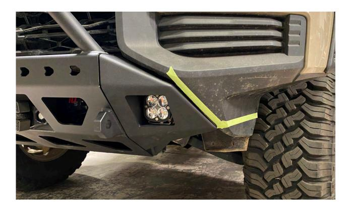
After tape lines have been laid along the sides place a tape line from the lower corner of the side flange parallel to the ground rearward toward the wheel as shown in the image. Our tape line and measurement for approximate cut location is shown in the image. Complete this process on both sides maintaining as much symmetry as possible. Now remove the bumper side flanges and then the main section to give room to complete the additional clean up and lower bumper plastic trimming.
