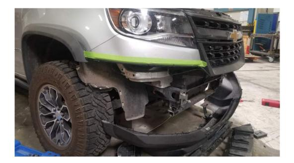
At this point we'll need to touch up, fine tune and sand down or cuts until smooth. See image below for an example of a finalized cut. We've sanded away the black plastic from the lower bumper until it just matches up with the colored portion, and cleaned up our cut at the bottom corners of the grille.
