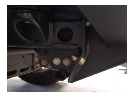
We are now nearly complete with the bumper installation. At this time re-check all fasteners to be sure they're installed tight.
