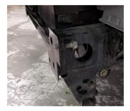
Now lift and position the bumper over the bolts loosely secure the bumper to the truck with the additional bolt into the frame end plates- these are accessed through the cutouts in the front of the bumper. Install the 2 factory skid bolts Begin to tighten the bolts in order to raise the bumper up. Adjust to about ½ inch clearance between top of plate bumper and lower edge of the plastic cut edge under the headlights as can be seen in the image below.
