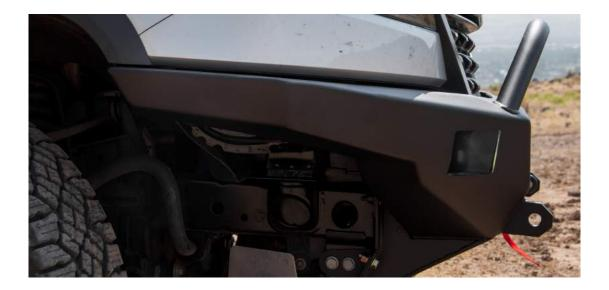
Once desired height is achieved and bumper is level side to side secure the 4) frame end bolts, taking the ones that were installed from the back of the plates to aid in bumper install, and reinstalling them normally from the front to secure the bumper. With these
