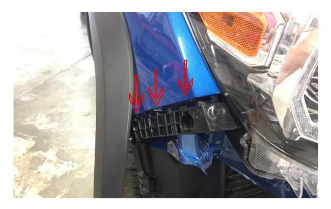
Work your way around to the other side, or with 2 people release each side simultaneously working from the outside by the fender flare in toward the center of the vehicle under the lights. Set the bumper cover aside being careful not to scratch it.
