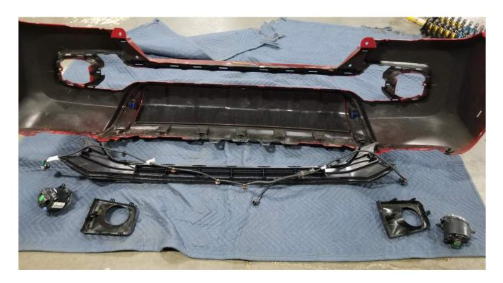
At this point we are now ready to lay out our cut line on the completely stripped down bumper cover. Using masking tape lay a cut line similar to the photo below.
