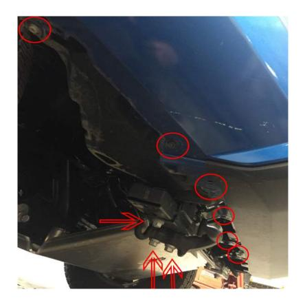
We need to release the sides of the bumper from the liner at the fender wells. Locate the fasteners and clips shown below. Remove the screws and pop the clips loose. After all have been loosened, free the bottom corners of the inner fender well liner, and then continue upward separating it slightly from the bumper cover as shown in the image. Separating the clip from the cover with a flat screwdriver may be helpful. Repeat for other side.
