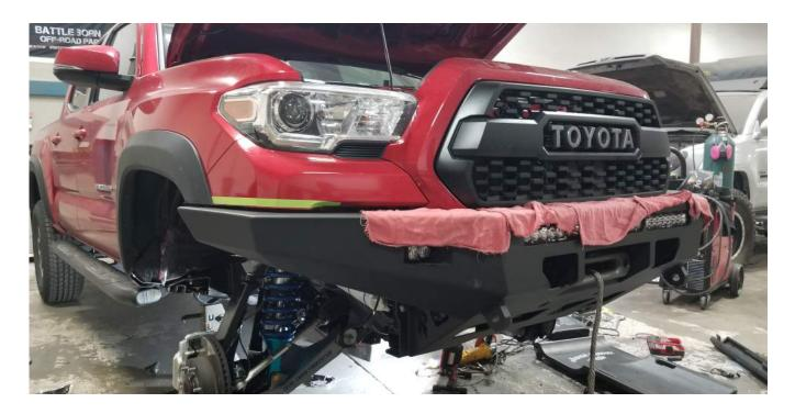
Installed bumper final gap. Make sure you have about 1/2" clearance between bumper and plastic bumper cover to allow body movement off road over bump and during articulation.
