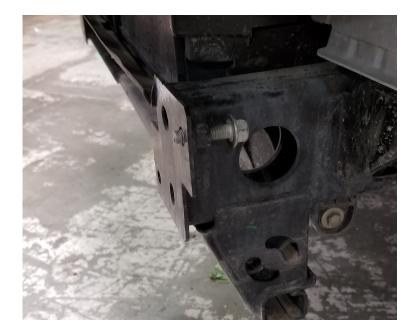
Now lift and position the bumper over the bolts loosely secure the bumper to the truck with the additional bolt into the frame end plates- these are accessed through the cutouts in the front of the bumper. Install the 2 factory skid bolts Begin to tighten the bolts in order to raise the bumper up. Adjust to about ½-5/8" clearance between top of plate bumper and lower edge of the plastic cut edge under the headlights.
