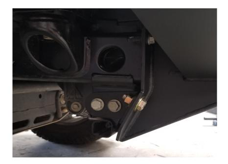
We are now nearly complete with the bumper installation. At this time re-check all fasteners to be sure they're installed tight.
