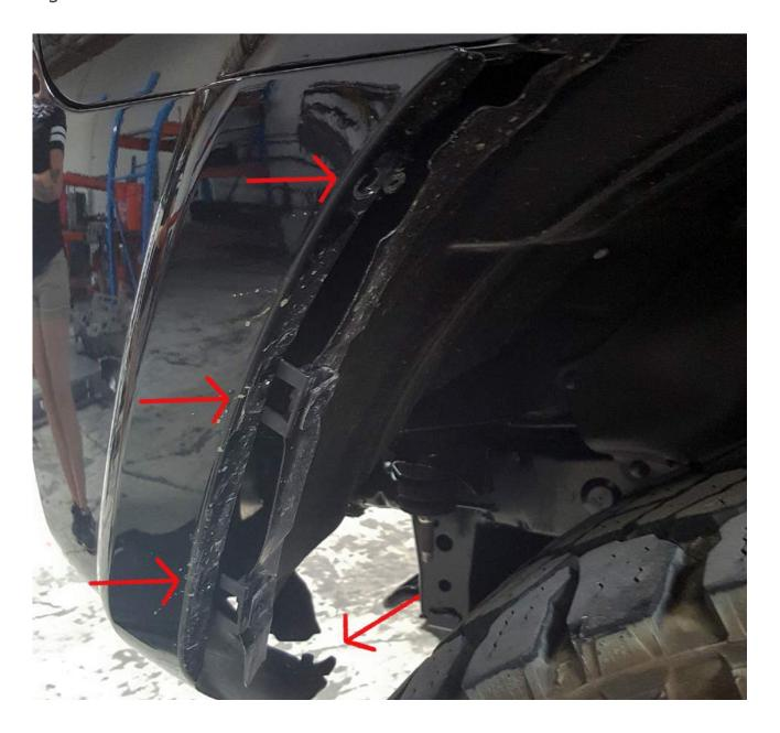
At this point we are now ready to remove the cover. The bumper cover is now only held on via some body clips along the upper edges under and near the headlights. Pull it lightly away from the body at the corner by the fender well (it it clipped over a shoulder at the upper screw the locations from Figure 3) and it should start to release.
