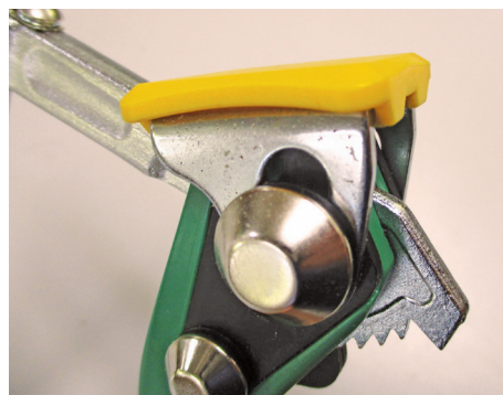
The swivelling head is liable to slipping
