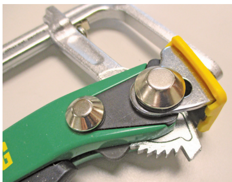
Close-up of the ratchet mechanism
