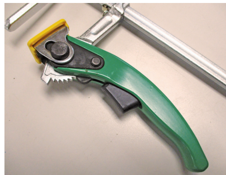
The ratchet lever provides power
