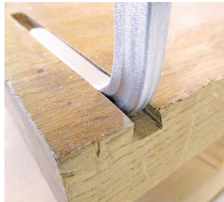
Both clamps use a standard 14° dovetail groove
