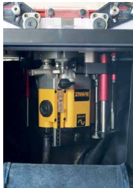
The router table fitted with the JessEm Rout-R-Lift Prestige
