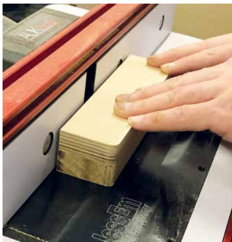
Following a template while routing small, intricate oak parts
