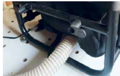
The router table features two large dust extraction ports with a downdraft bag
