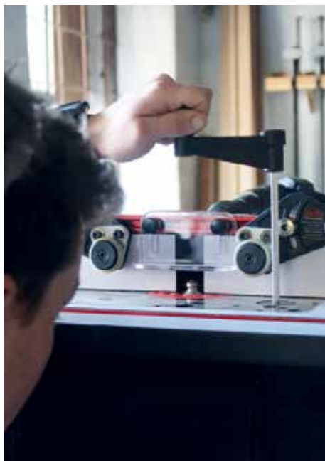
Using the Rout-R-Lift enables easy and precise router height adjustment
