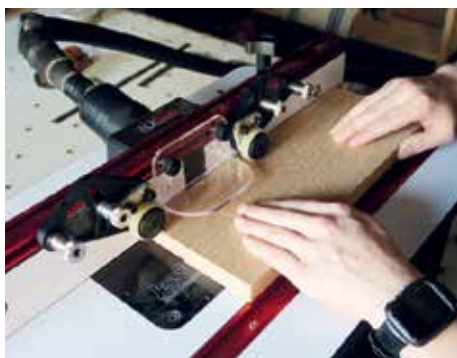
Dust extraction is excellent while routing a rebate in solid oak
