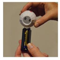
When replacing the battery compartment, make sure that the two pins line up with the metal points inside the globe. The metal strip on the side of the battery compartment must line up with the groove inside of the Globe Light.
