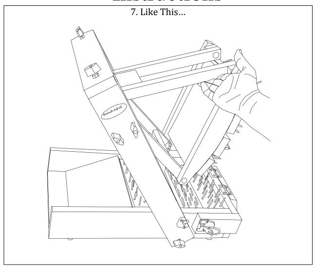
8. Clasp the rocker frame latches, holding the picker in the upright position.
