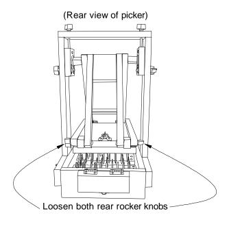
3. Slightly loosen *both* of the rocker frame knobs. There's a knob on both the right and left side of the picker, at the base.
