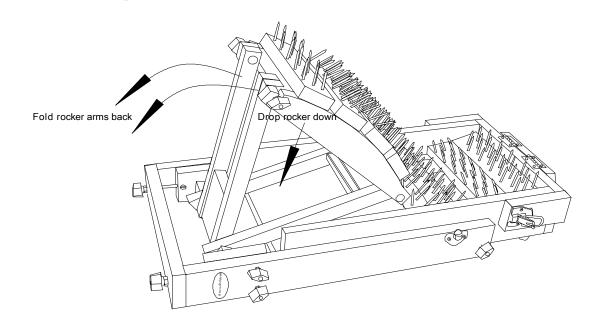
7. First, lift rocker up and fold it down into the bottom bed of teeth, then fold the rear rocker arms down.
