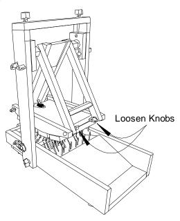
2. Loosen both rear rocker knobs.
