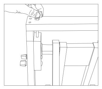
3. Begin by lining the top of the adjustment *boards* even with the basic adjustment *lines* as shown. The basic adjustment line is a recommended adjustment for medium wools. To further adjust wool picker to your own specifications, simply rotate the two adjustment knobs equal number of turns to raise or lower the rocker.
