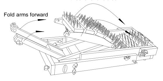
8. Fold the safety latch board up to the rocker as shown.
