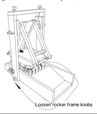
4. Unclasp both rocker frame latches. (One on each side of the picker.)
