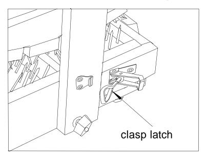
As you use your picker it will develop a slight forward and backward movement of the top of the picker. This is normal, and won't affect the picking process. If you wish to reduce this movement simply unclasp latch and rotate the latch screw clockwise ½ turn, and reclasp. (Repeat on other side).
