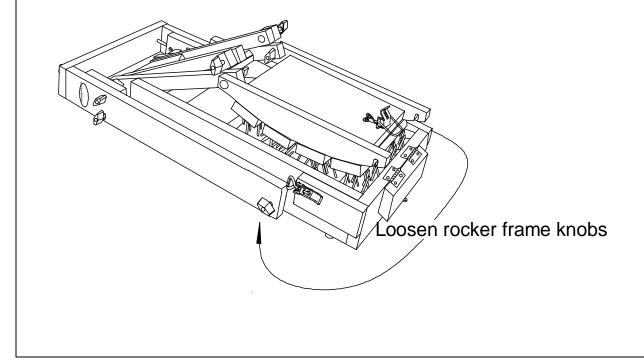
3. First fold the top two rocker arms up and back, then fold the rocker up.
