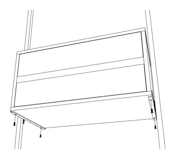
Tip: Attach dresser with supports higher up. Once dresser is attached, move the dresser with brackets further down in preferred position
