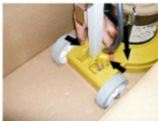
Step 7-Put screw protector back onto the chassis.
