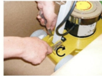
Step 6- Insert the screw and tighten the nut.
