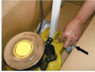
Step 5-Align the mounting hole of the handle assembly with the mounting hole of chassis.
