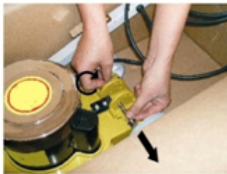
Step 4- Remove the Handle Assembly and the Screw.
