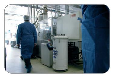
The R series is specifically designed for use in packaging applications in industries such as food and pharmaceutical. The features of these vacuums make it ideal for removing excess lateral trim and scraps during packaging processes.
