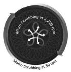
Patent-pending REV random orbital scrubbing technology with high speed ¼ inch micro scrubbing and 20 inch rotational macro scrubbing attacks dirt from multiple directions for superior cleaning effectiveness.
