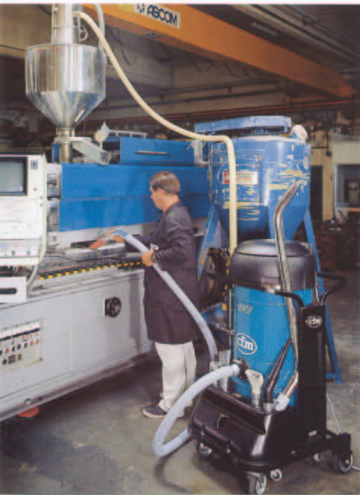
PLASTIC INDUSTRY Sucking of granules, dust and oil
