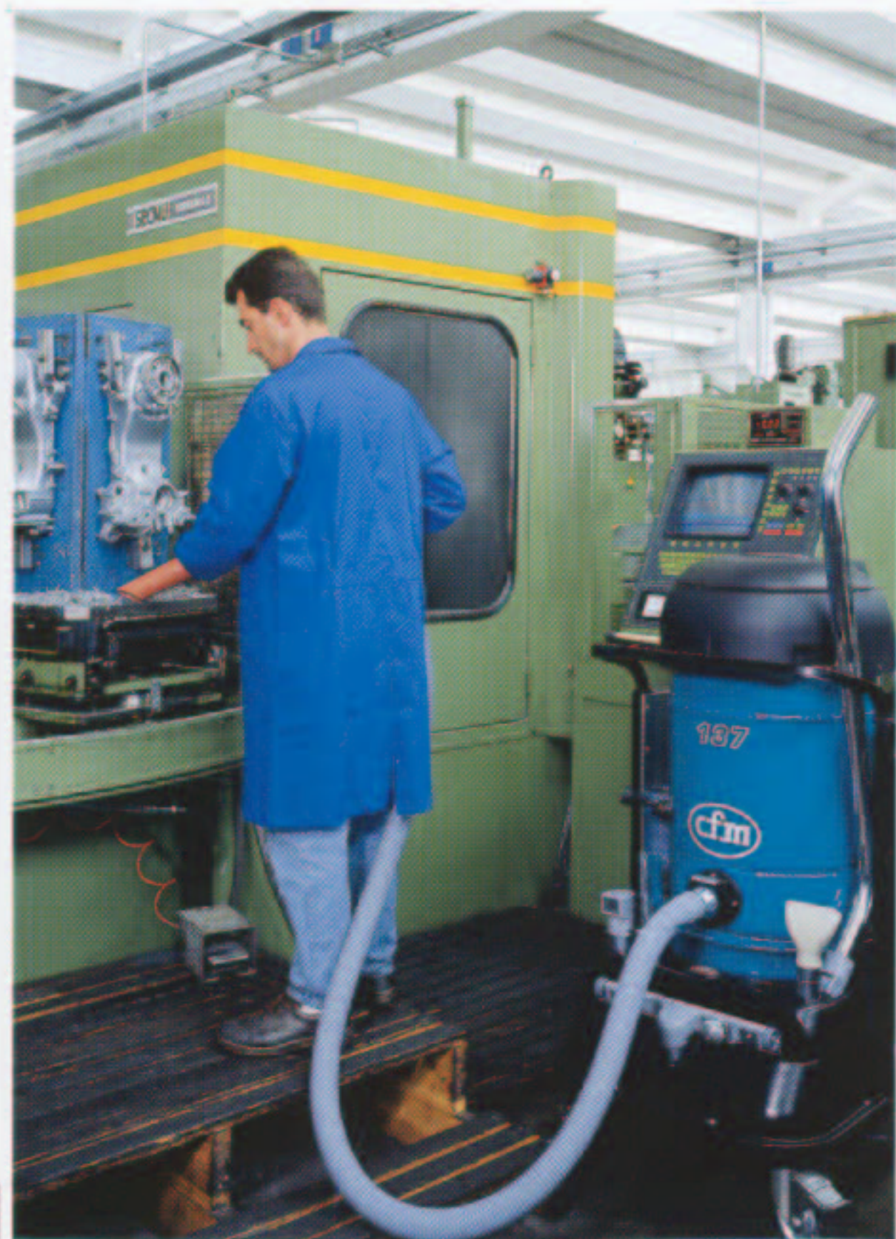
METALWORKING INDUSTRY Vacuuming of waste from boring machine
