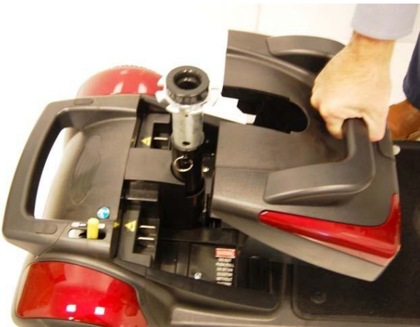
Figure 21: Battery Pack Installation
