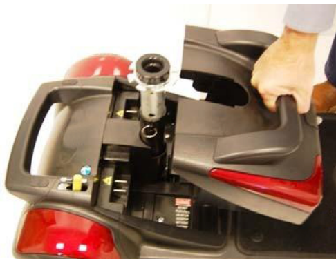
Figure 15: Removing the Battery Pack
