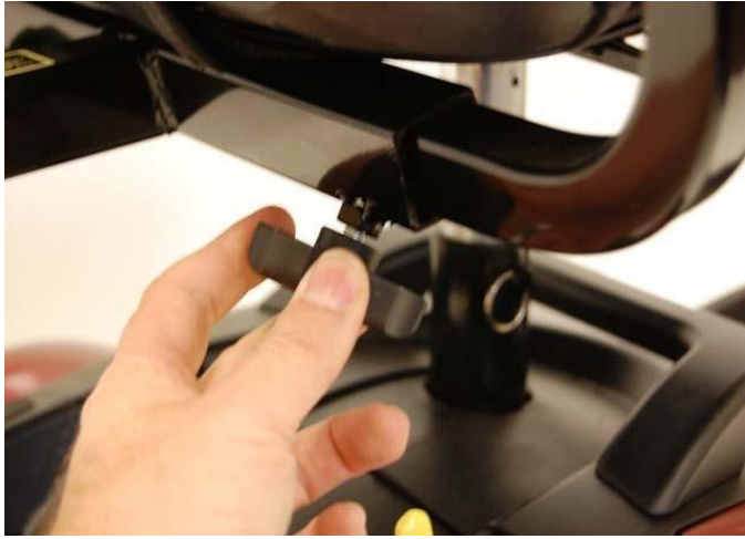
Figure 6: Armrest Width Adjustment
