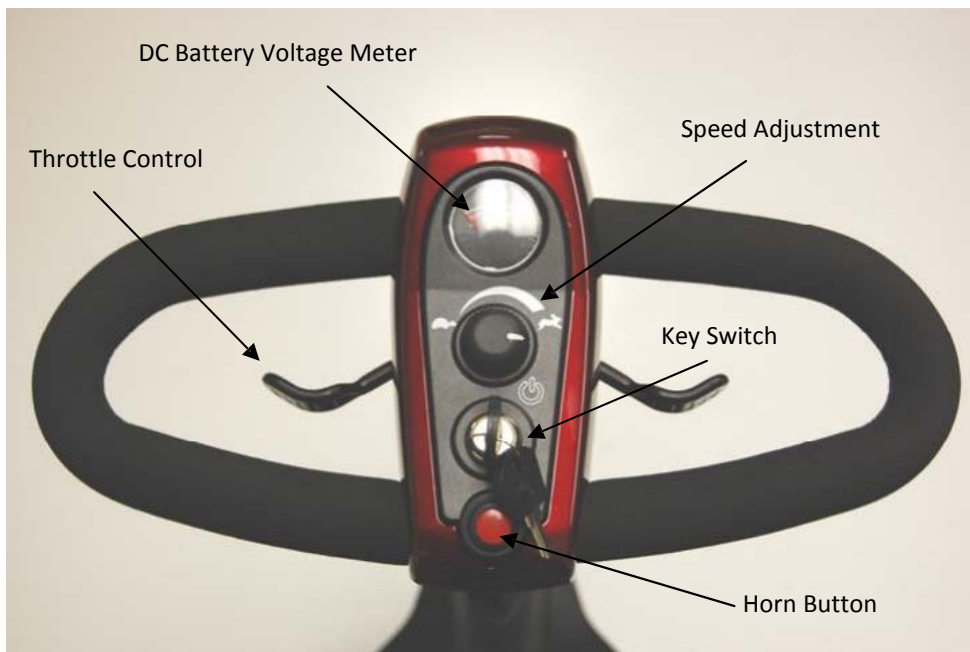
Figure 5: iGO COMPACT Delta Tiller Control Panel
