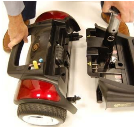
Figure 20: Connecting Frame and Drivetrain
