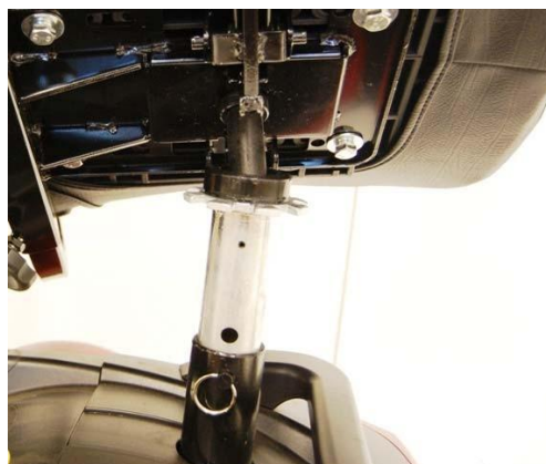
Figure 23: Installing the Seat
