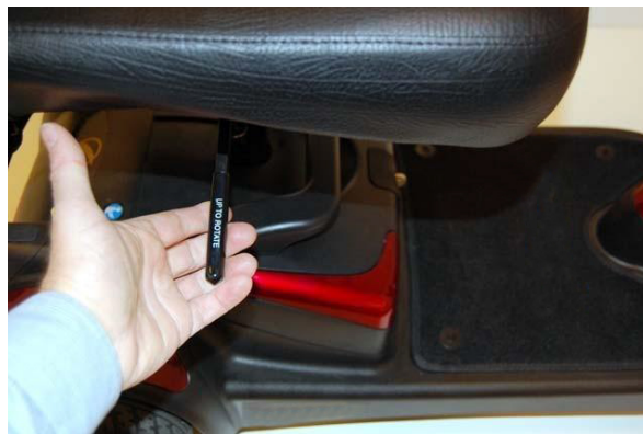
Figure 8: Seat Height/Rotation Adjustment
