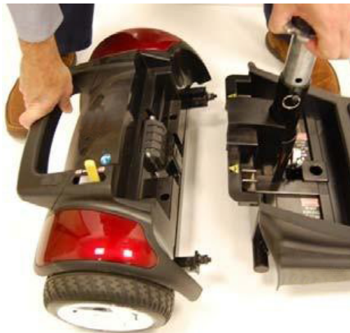
Figure 17: Releasing the Drivetrain
