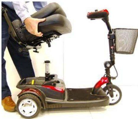
Figure 14: Removing the Seat
