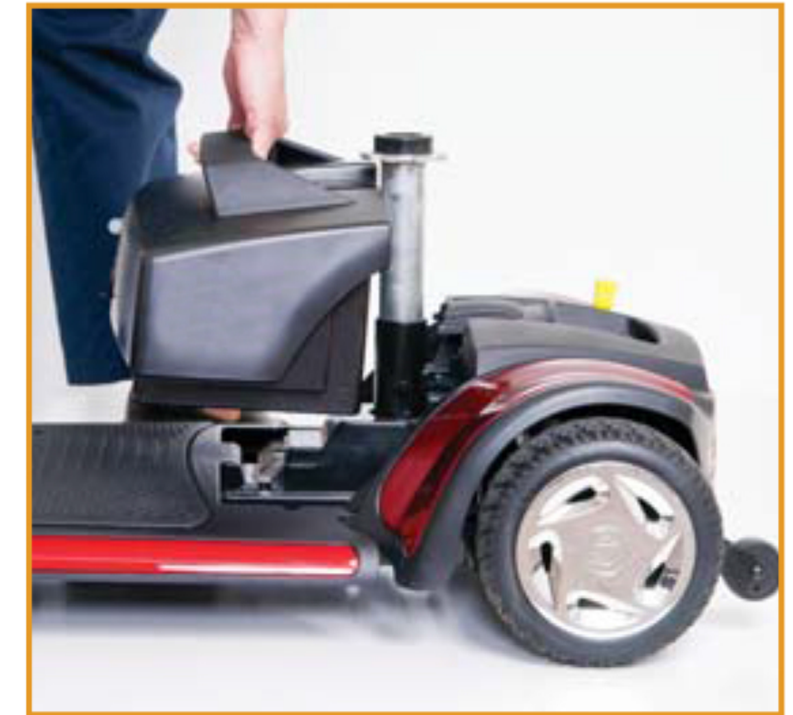
Step 2: Pull out the battery pack!
