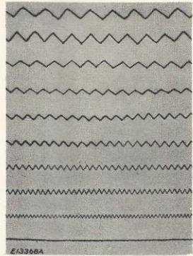
Fig. 5. Illustrating Different Shapes of Zigzag Stitch Produced by Varying the Length and Width of the Stitch
