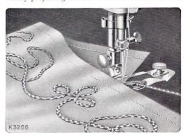
hole in the throat plate at the right of the feed dog. Then place the guide thumb screw in the slot of the attachment and into the hole in the bed plate of the machine. The under braider must be firmly secured by tightening the screw.
