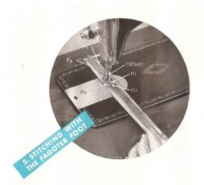
Attach the Fagoter Foot (H) to the Presser Bar with the reg-ular thumb screw. This screw is placed in the upper hole in the shank of the foot on Singer 101 Machines. On all other Singer lock-stitch family machines, the screw is placed in the lower hole of the foot.
