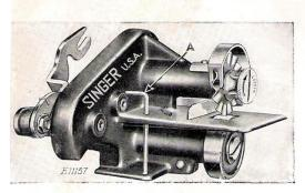
Fig. 1. Rear View of Pinking Attachment
