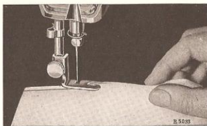
FIG. 84. STARTING A HEM AT THE EDGE
