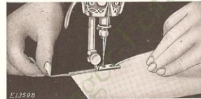
FIG. 85. MAKING A HEM WITH THE FOOT HEMMER
