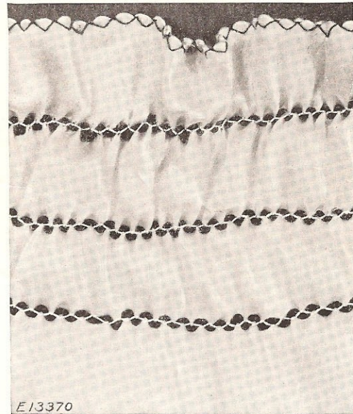
Fig. 12. Cording with Slight Gather, also Purl Effect on Rolled Seam.
