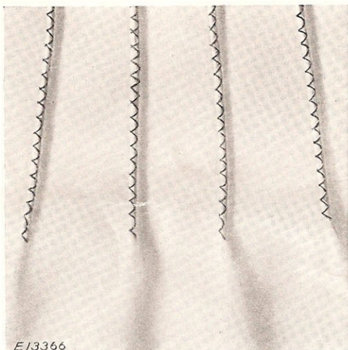
Fig. 11. Narrow Cord-Like Tucking Produced with Zigzag Attachment.
