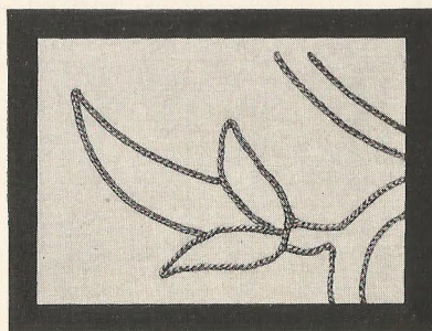
FIG. 197. WORK DONE BY THE BRAIDING PRESSER FOOT
