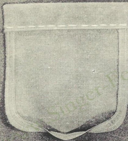
Patch Pocket prepared for Application
