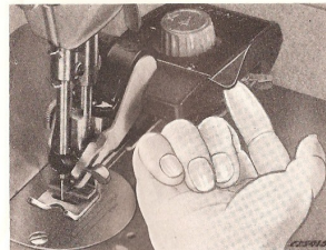
Fig. 7. Lifting Cover to Remove Stitch Pattern
