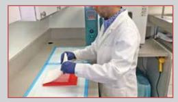
Step 4: Roll over the mold to unfasten the compounds off the mold
