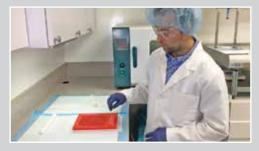
Step 3: Bend, flip, and remove the white bottom component of the mold
