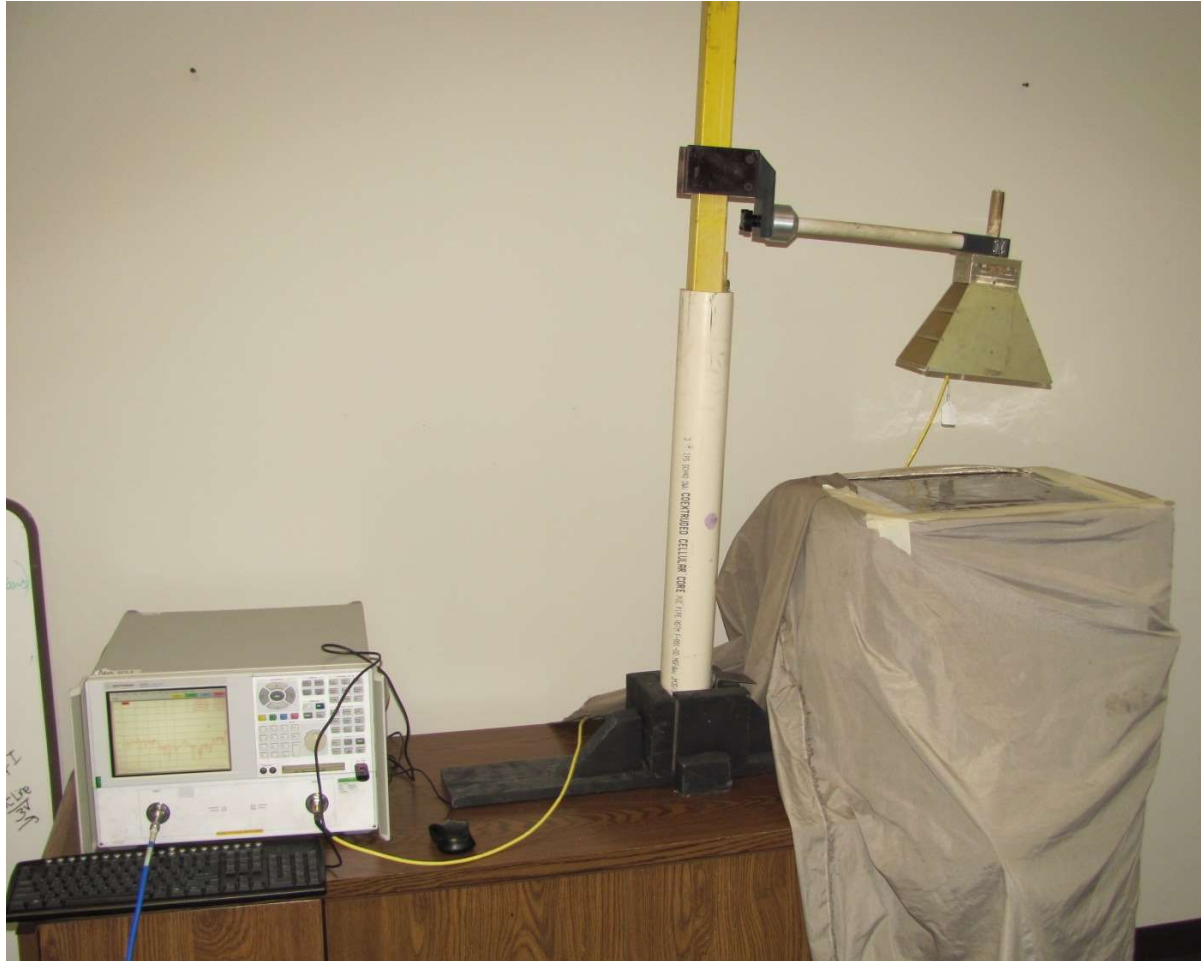
Figure 6. Sample Under Test Sealing Enclosure Opening – Above 6 GHz Testing
