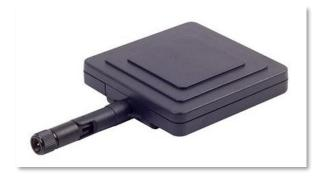
The directional patch antenna is a high gain, excellent choice to use RF Explorer analyzer to scan in a specific direction. As opposed to omnidirectional antennas such as dipole type, this patch antenna has an 8dBi gain in the front face. It includes a true SMA connector (not RP-SMA as most in the market) and therefore fits perfectly in all RF Explorer models.
