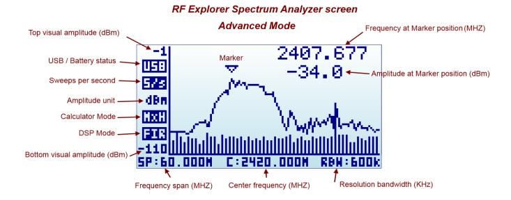
Note the frequency axis indicators changes at the bottom. More details about this screen mode in section *Analyzer screen* page 18.
