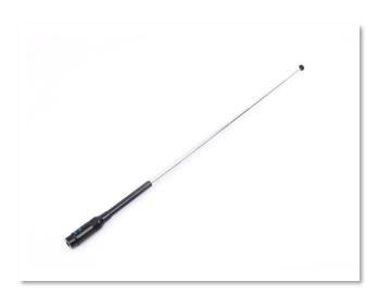
It offers a good response in all frequencies below 1GHz. Use this antenna in all ranges of frequencies between 15-1000MHz. In some cases, collapsing partially or totally may provide better response in the highest frequencies of the range.
