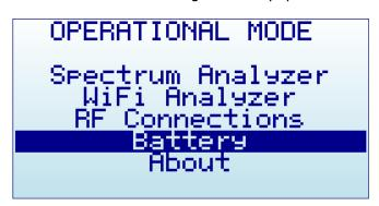
Inside this INTERNAL BATTERY charger screen, it is easier to realize if the battery is being charged. In this case below, it clearly indicates the power switch is not in the ON position and, therefore, battery is not being charged.
