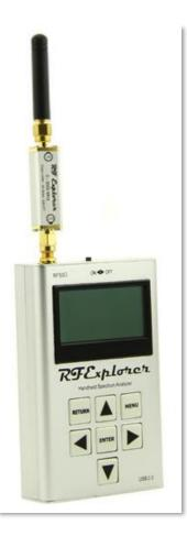
The RF Explorer Power Limiter will allow any RF Explorer model to be protected with external signals up to +30dBm (1 Watt), so you get the same level of protection as in the WSUB3G. Furthermore, the power limiter includes additional functionality inside that will otherwise require external devices increasing cost and size:
