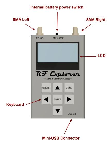
The RF Explorer Standard models includes 7 functional buttons in the front side. The unit also includes at least one RF connector 50 ohm impedance standard SMA format.
