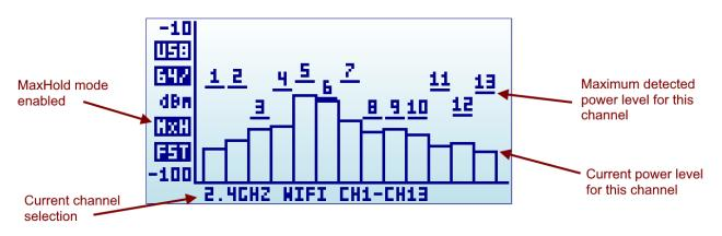
Use [RETURN] button to recycle a MaxHold capture Use [LEFT]/[RIGHT] buttons to cycle through available channels (only in 6G Combo/PLUS models)
