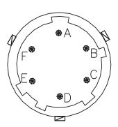
8-pin connector PC02E-12-8P Bendix
