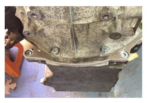
10) Now you can install your starter. Using the two M10x1.5 45mm long flange head bolts, attach the starter to the adapter/transmission.
