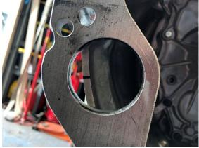
4) Remove the adapter plate and use a ruler to mark 5/8" above and below the mark made in the previous step. These will be the upper and lower limits of your notch. Then mark the side of the bellhousing 5/8" back from the front edge. Using your ruler mark a rectangle connecting those dots. This is the boundaries of material that needs to be removed.
