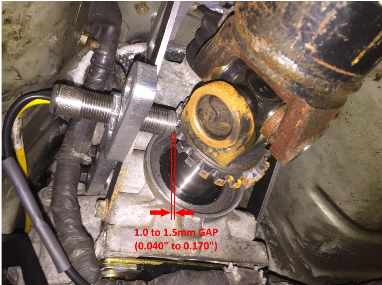
8. Once the gap is set, use a wrench to tighten the jam nut to lock the sensor in place. To prevent the sensor from turning, you can hold the knurled end of the sensor with a pair of channel-lock pliers.
