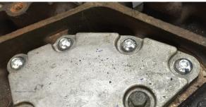
3) Install the LOJ Conversions Transmission Adapter Plate onto your Engine. Use four M10x1.5 30mm Low-Profile Socket Head Cap Screws and four M10x1.5 35mm Flange Head Cap Screws. If your engine did not have alignment dowel pins, install them before installing the adapter plate! Additionally, if you are using an aftermarket oil pan that does not utilize the lower two bolt, leave them uninstalled.
