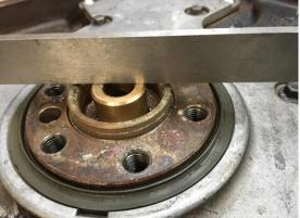
2) First you will need to replace the top four bolts holding the rear cover onto your engine. This is necessary to provide clearance for the transmission adapter plate. Use the four supplied M8x1.25 25mm long button head allen key bolts. Replace the bolts one at a time to prevent unsealing the gasket.
