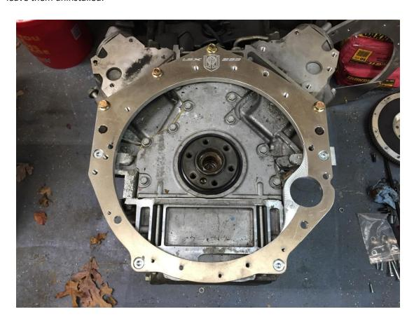
4) You will need to remove one boss from the RH rear side of your engine to provide sufficient clearance for the new starter. This can be accomplished with an angle grinder, hack saw, sawzall, or other suitable cutting tool.
