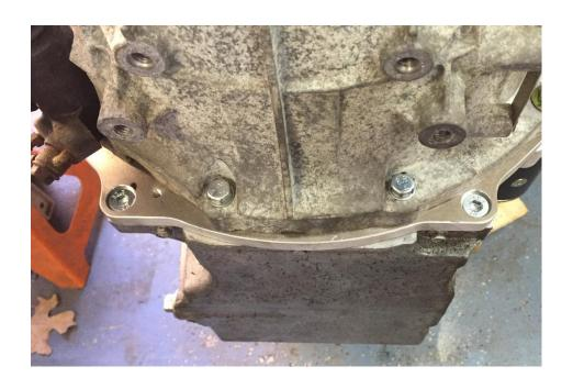
8) Now you can install your starter. Using the two M10x1.5 45mm long flange head bolts, attach the starter to the adapter/transmission.
