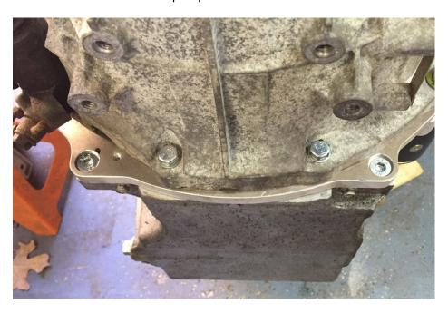
9) Now you can install your starter. Using the two remaining M10x1.5 55mm long bolts with flat washers, attach the starter to the adapter/transmission.
