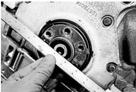
2) First you will need to replace the top four bolts holding the rear cover onto your engine. This is necessary to provide clearance for the transmission adapter plate. Use the four supplied M8x1.25 25mm long button head allen key bolts. Replace the bolts one at a time to prevent unsealing the gasket.
